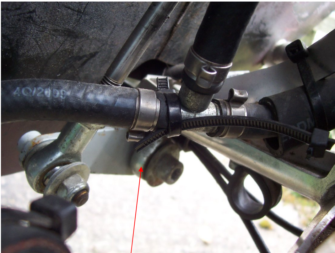
Aft Control tube bearing
