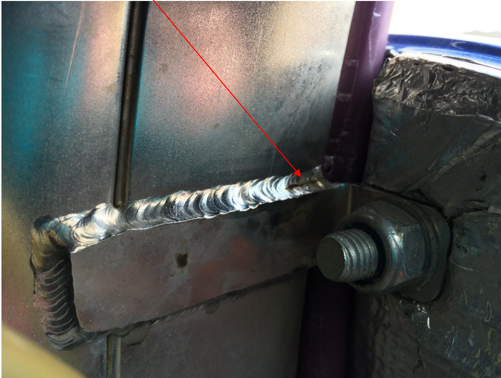
Crack in left-hand bracket
