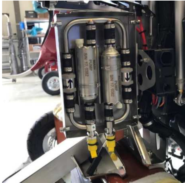
Figure 1 - Location of pumps inside the Rotax pump box (915 engine)
