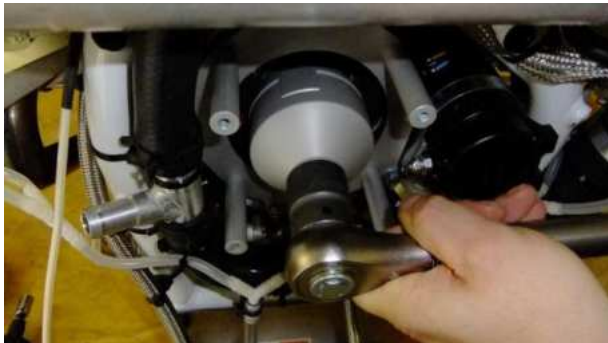
Figure 5 – Torque Dog Gear with 140 Nm
