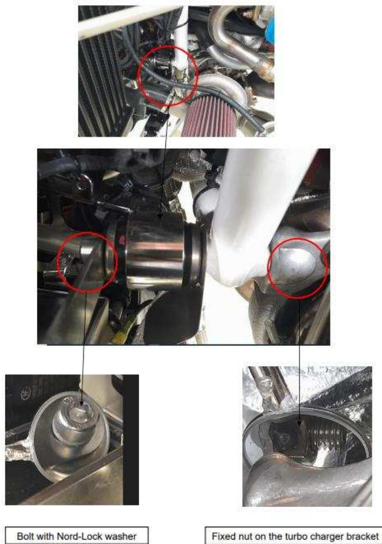
Figure 3 – 915 / 916 version with fixed nut
