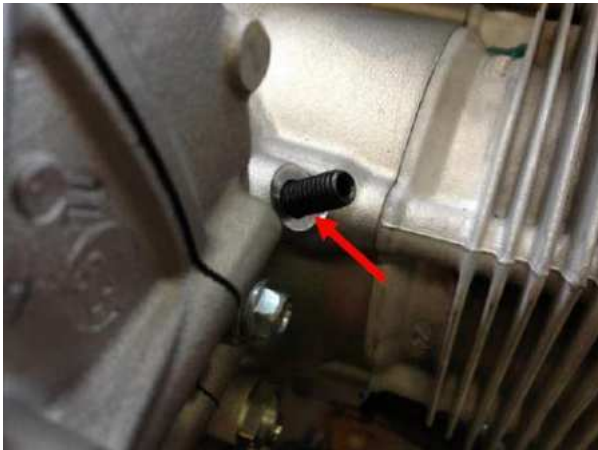
Figure 3 – Thread Pin M8 x 50
