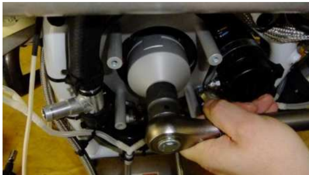
Figure 5 – Torque Dog Gear with 140 Nm
