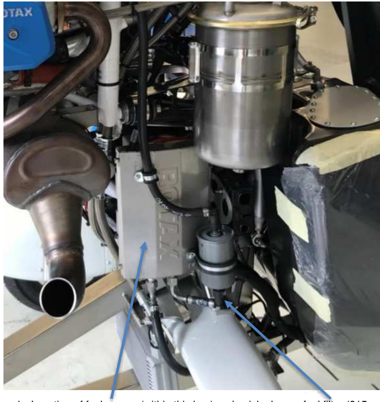
Figure 1 - Location of fuel pumps (within this box) and quick-change fuel filter (915 engine)
