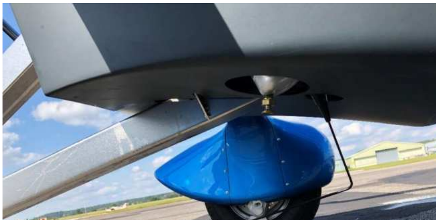
Location of gascolator drain point
