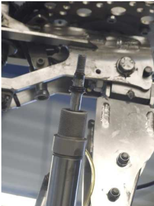
Figure 3 - New seal ring installed with special grease
