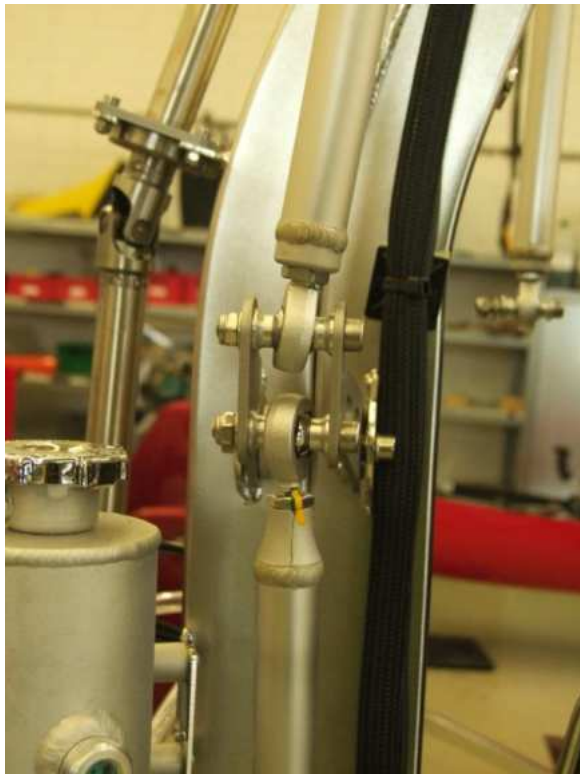
Figure 2 - Connection of upper ball joint of lower RH flight control rod with bell crank(step3/5)
