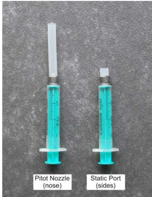
Figure 1 – Pitot Static Integrity Test Equipment Pitot Nozzle
