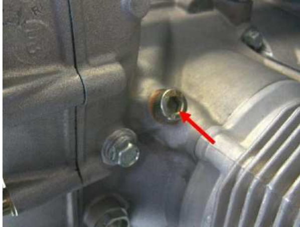
Figure 2 – M8 x 20 Screw Plug
