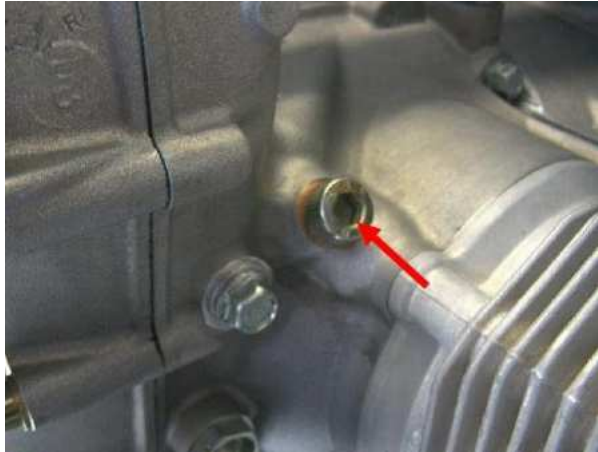
Figure 2 – M8 x 20 Screw Plug
