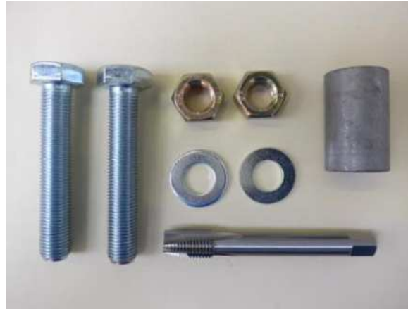
Figure 4: Bushing removal tool Teeter Block
