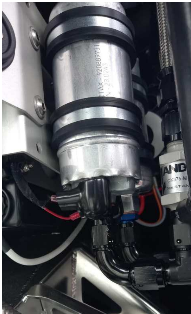
Figure 2 - Electrical fuel pump (916 engine)
