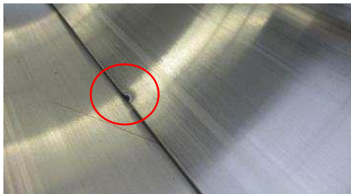
Figure 4 – damage on trailing edge
