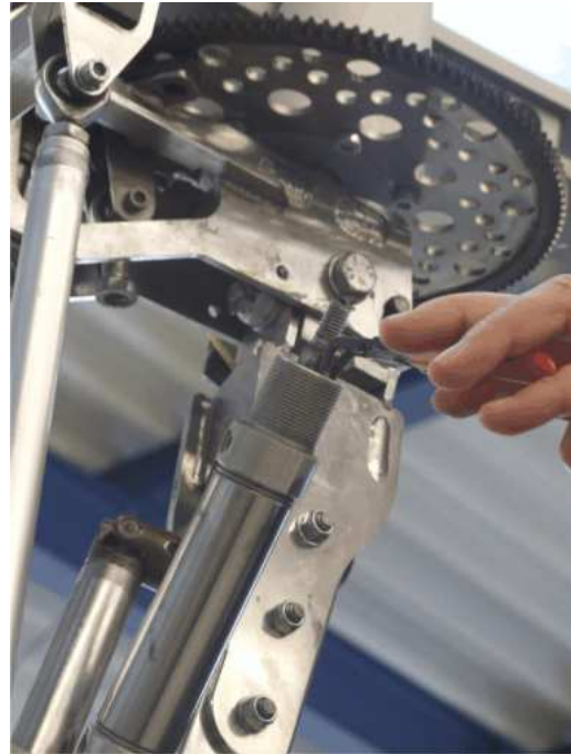
Figure 2 - Remove circlip / snap ring
