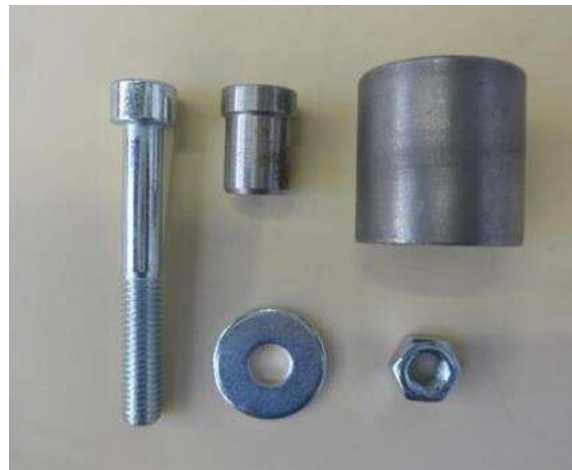
Figure 5: Bushing removal tool for Teeter Tower
