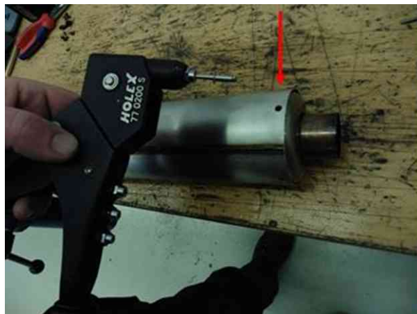
Fig. 6 - Riveting of the outer shell
