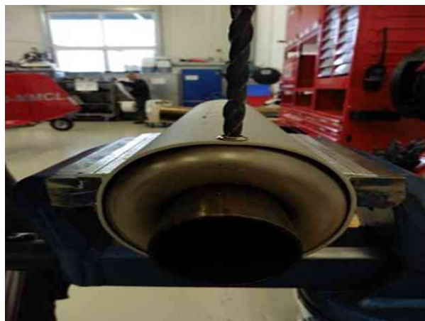
Fig. 3 - Drill out the rivet pin
