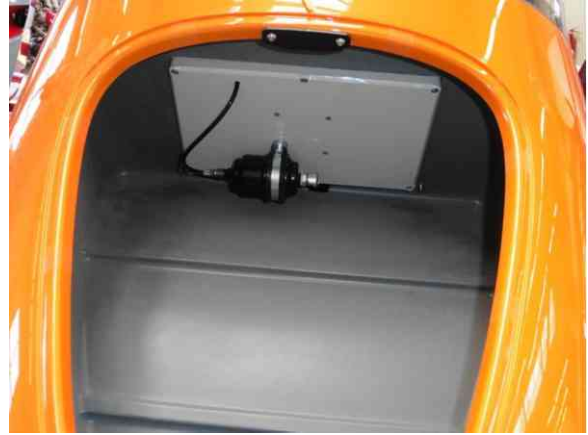
Fig. 1 - Access to dryer / nose compartment opened
