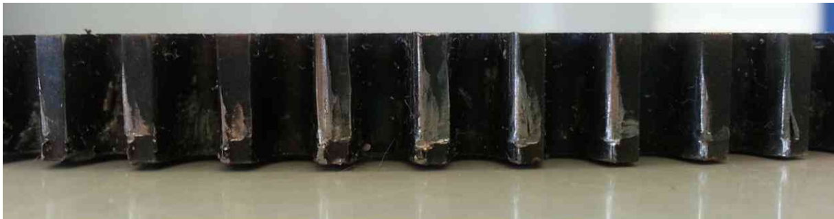
Fig. 1 - Wear Pattern (uneven)
