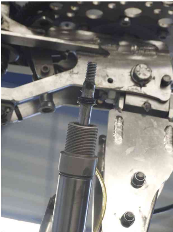
Fig. 3 - New seal ring installed with special grease (step 8)
