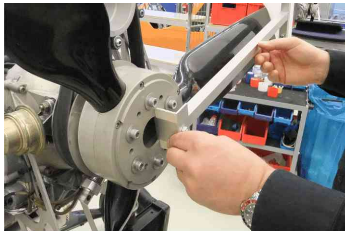
Fig. 2 - Propeller pitch adjustment and tool
