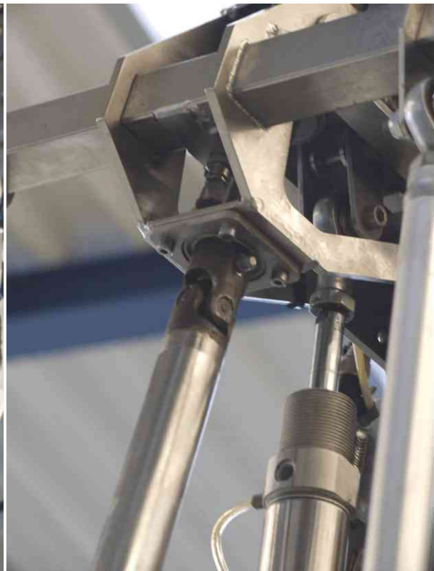
Fig. 4 - Re-connect ball joint and upper cardan hinge
