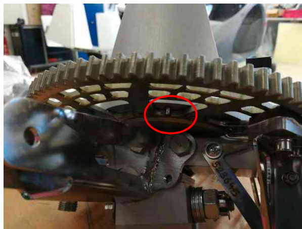
Fig. 3 - Hole or magnet in the 7 o'clock position in flight direction
