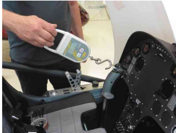
Fig. 1 - Measurement of rotor control friction
