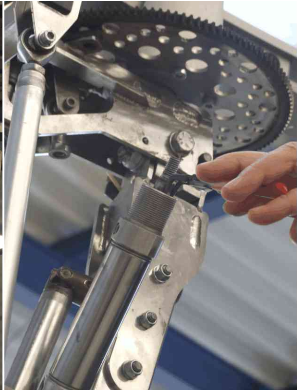
Fig. 2 - Remove circlip / snap ring (step 6)
