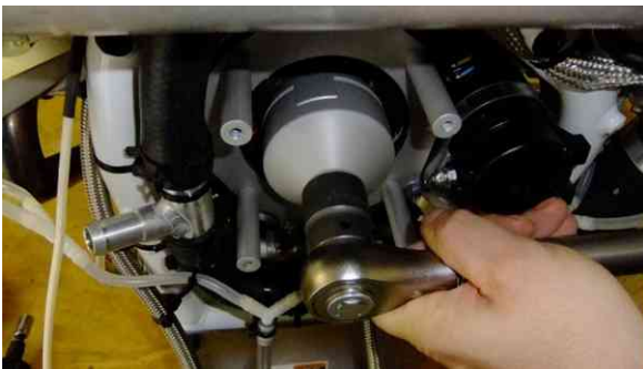
Fig. 5 - Torque dog gear with 140 Nm
