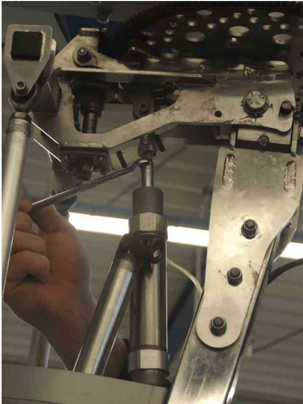
Fig. 1 - Disconnect rod end from ball joint (step 4)
