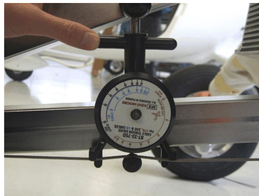
Fig. 3 - Measurement of control cable tension
