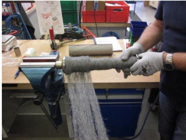
Fig. 4 - Installation of absorption wool
