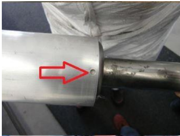
Fig. 5 - Rivets at the cold end of muffler tube
