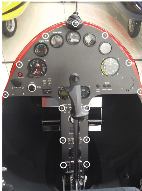
Fig. 3 - Instrument Panel with attachment bolts
