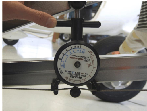
Fig. 3 - Measurement of control cable tension
