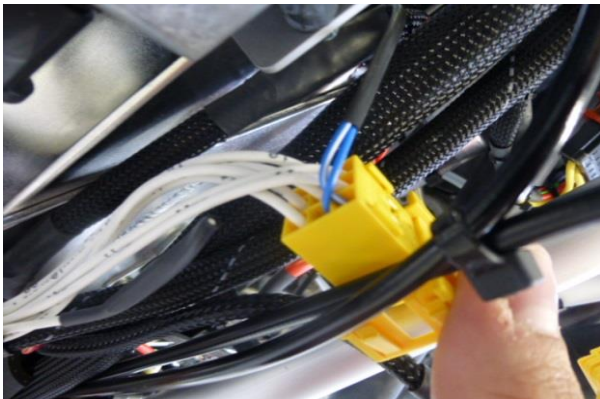
Fig. 8 – Turbo wires / pump wiring harness
