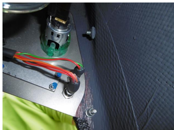
Fig. 6 - LEDs seen from behind
