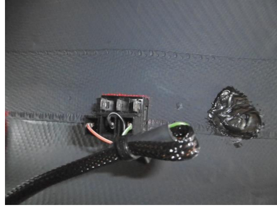
Fig. 8 - Connected rocker switch from below
