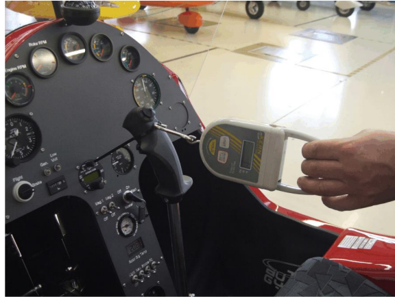
Fig. 1 - Measurement of rotor control friction
