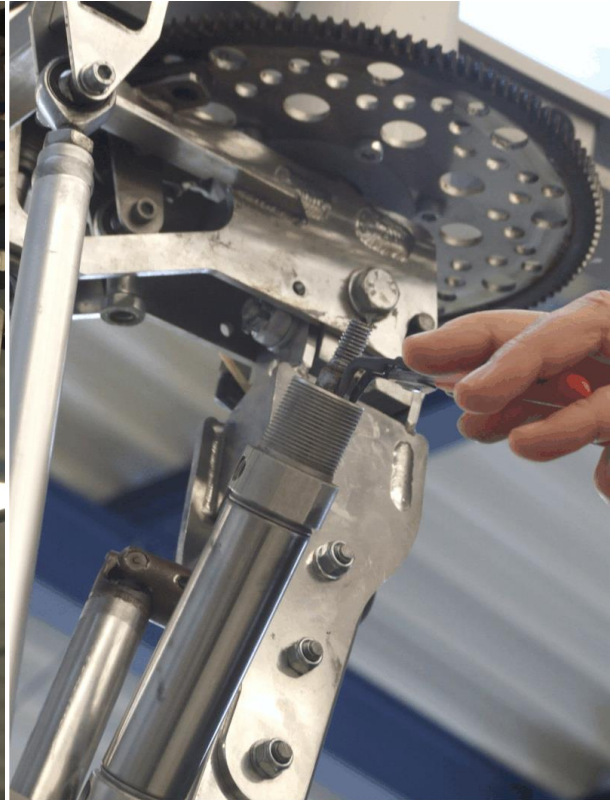
Fig. 2 - Remove circlip / snap rind (step 6)
