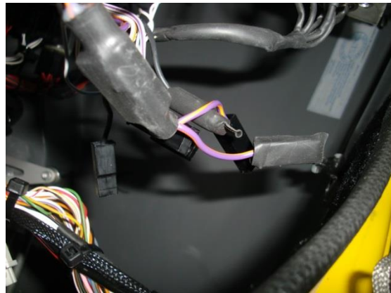
Fig. 4 - Isolation of cable end
