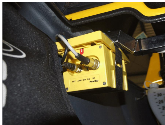
Fig. 2 - ELT transmitter below forward seat support frame on RH side
