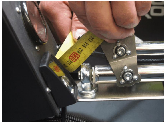
Fig. 3 - Fuselage reference point
