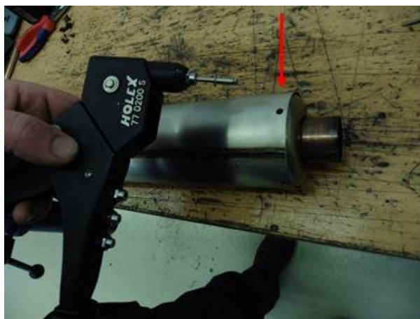
Fig. 6 - Riveting of the outer shell
