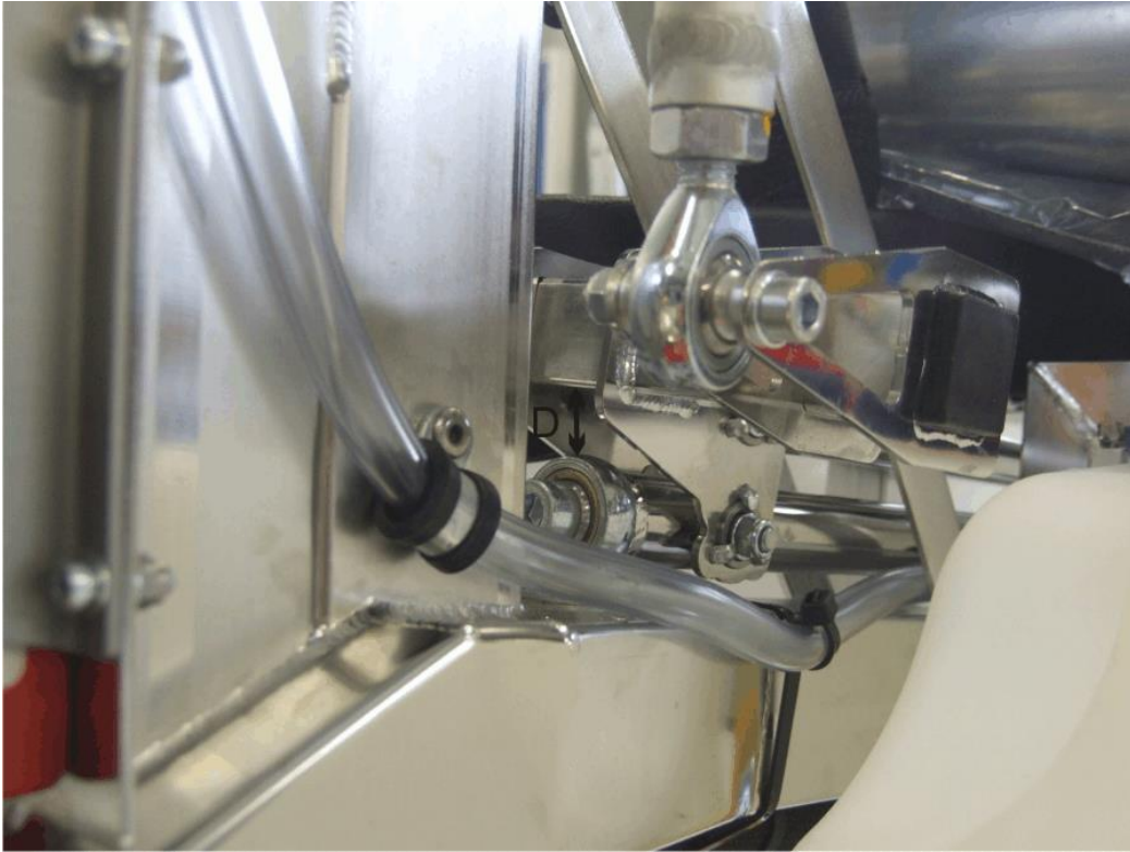
Fig. 1 - Clearance in flight control base link
