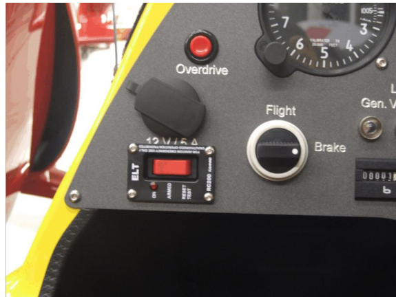
Fig. 1 - ELT remote control in instrument panel
