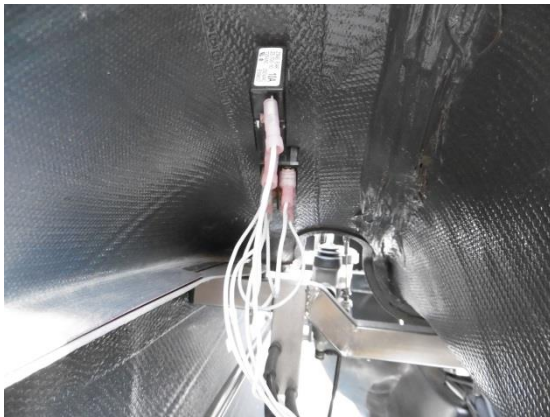
Fig. 3 - Rocker Switch - seen from below
