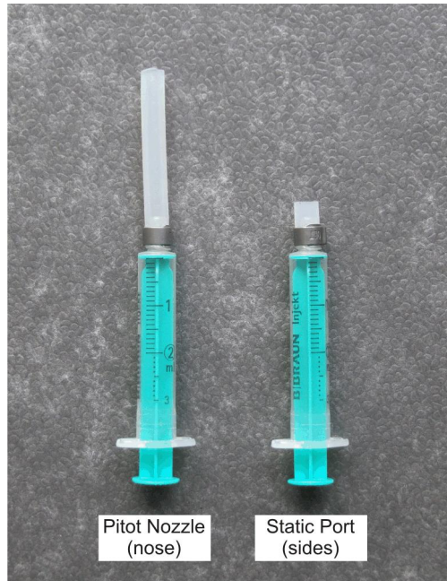
Fig. 1 - Pitot Static Integrity Test Equipment
