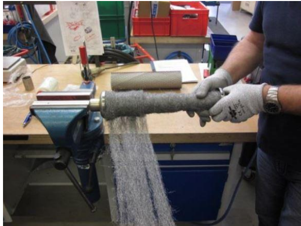
Fig. 4 - Installation of absorption wool
