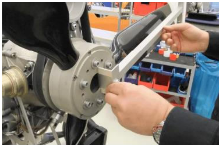
Fig. 2 - Propeller pitch adjustment and tool
