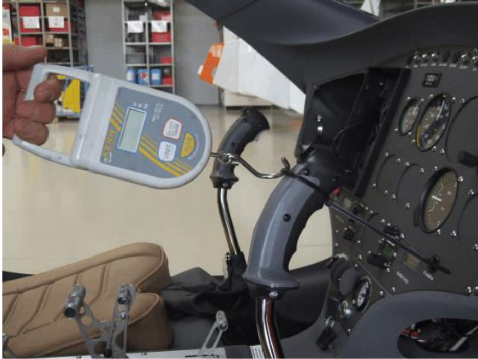
Fig. 1 - Measurement of rotor control friction
