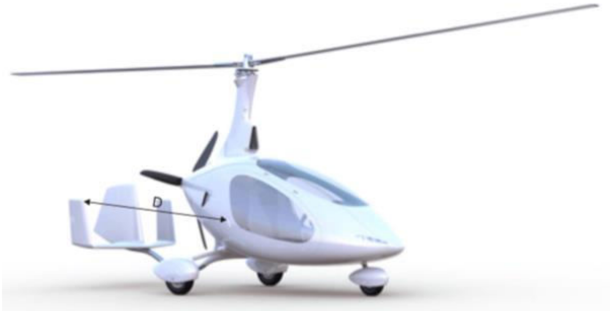
Fig. 1 - Measurement of Stabilizer Alignment (RH side shown)
