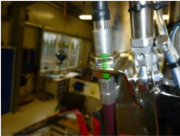
Fig. 2 - Push-pull control cable bulkhead attachment
