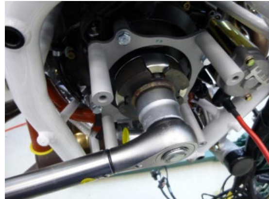
Fig. 4 - Tighten dog gear to 150Nm
