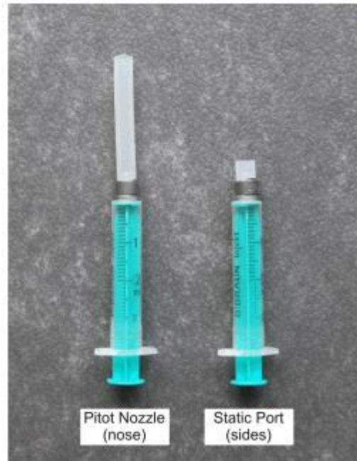
Fig. 1 - Pitot Static Integrity Test Equipment
