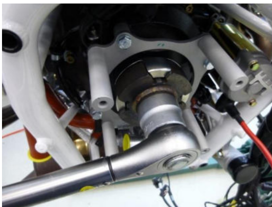
Fig. 5 - Torque dog gear with 150 Nm
