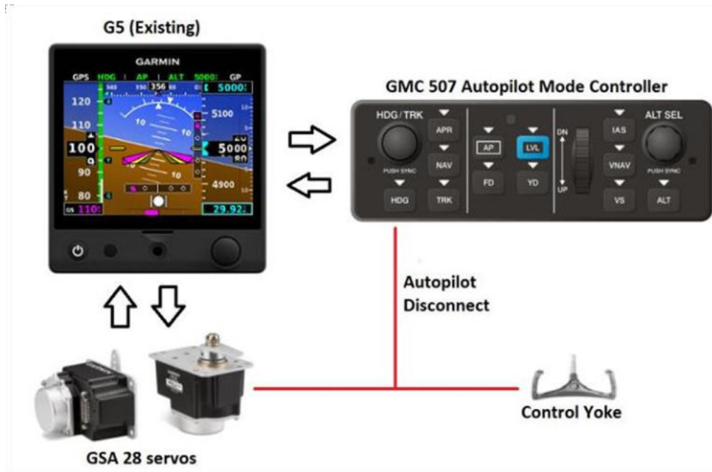
Figure 22-2 – GFC 500 System Overview
