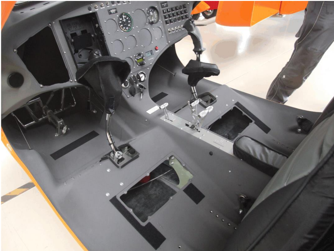
Fig. 1 - Service covers below seats ('Equipment Cover')
