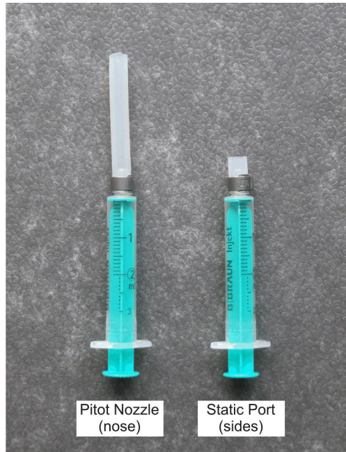
Fig. 1 - Pitot Static Integrity Test Equipment
