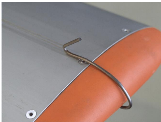
Fig. 2 - Positioning of measuring cord
