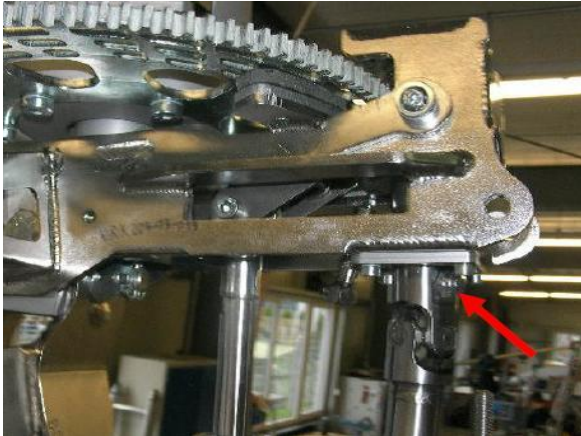
Fig. 1 - Upper pre-rotator drive connected to Bendix shaft
