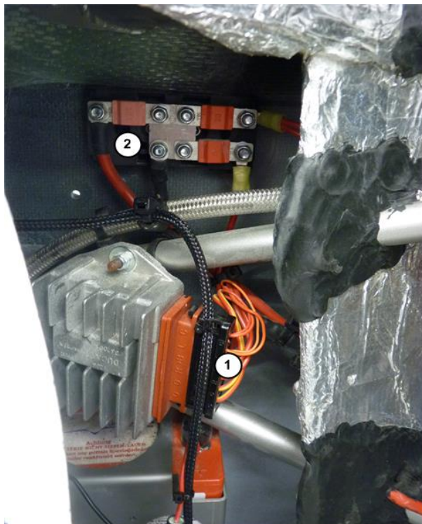
Fig. 1 - Cable connector on rectifier-regulator (1) and fuse carrier (2)
