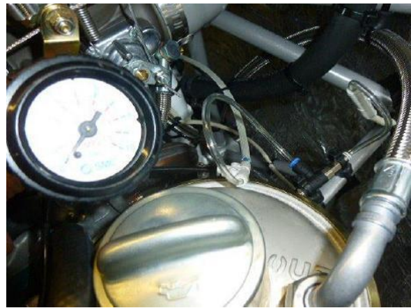
Fig. 4 - Connection between clutch and pressure reducer
