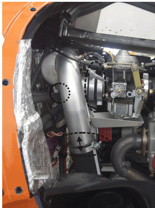
Fig. 1 - Clearance airbox to engine mounting frame (R914)
