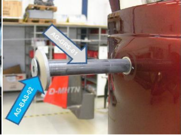
Fig. 7 - Installation of mast bushes
