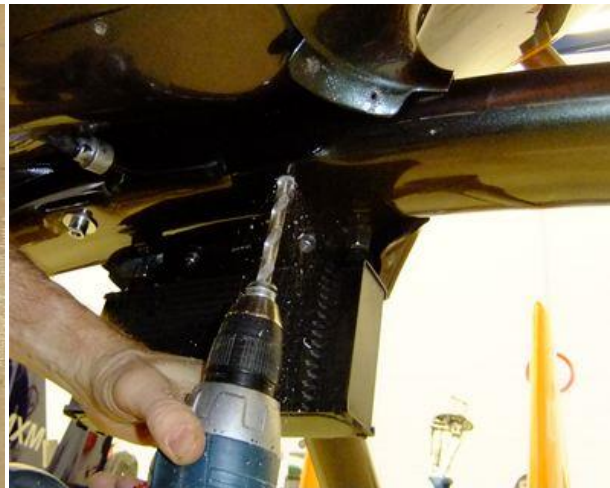
Fig. 4 - Drilling to a diameter of 10 mm
