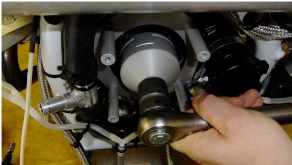
Fig. 5 - Torque dog gear with 140 Nm
