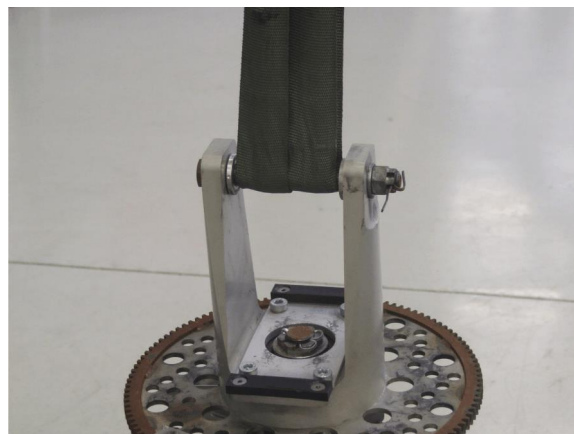
Lifting belt looped around teeter bolt
