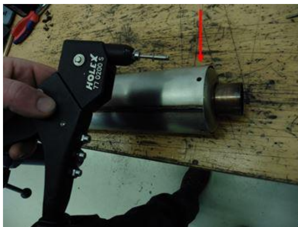
Fig. 6 - Riveting of the outer shell
