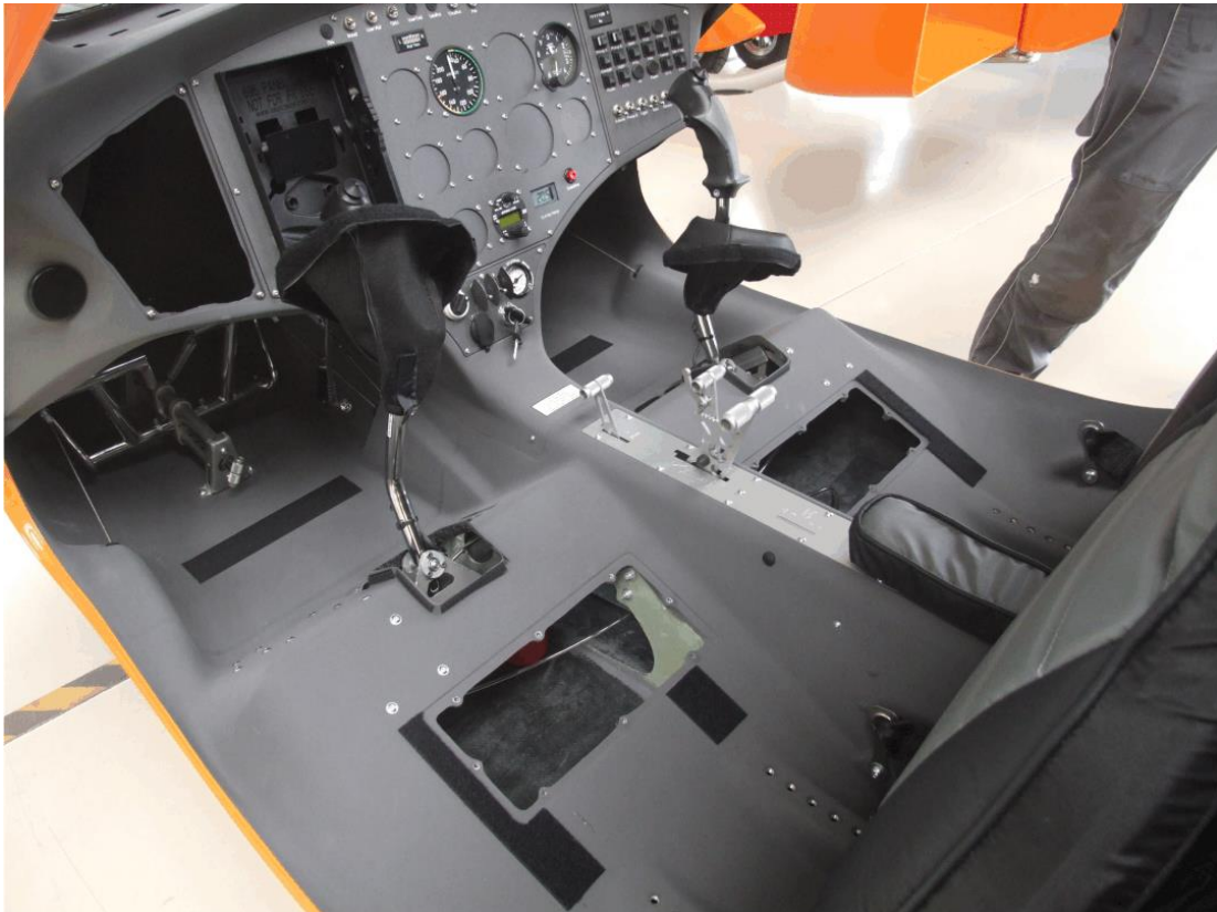
Fig. 1 - Service covers below seats ('Equipment Cover')
