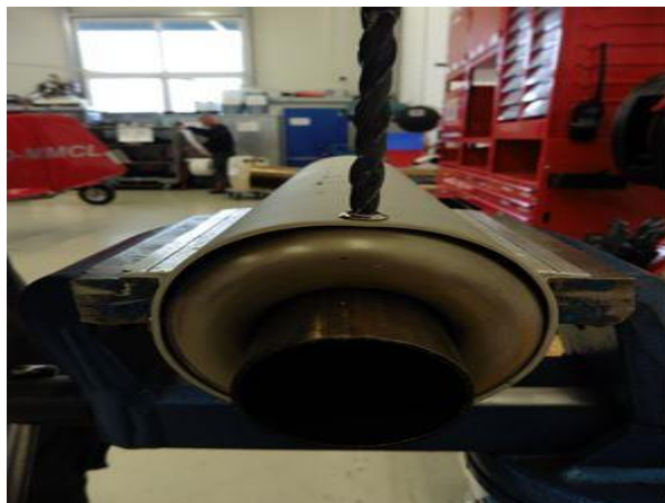
Fig. 3 - Drill out the rivet pin
