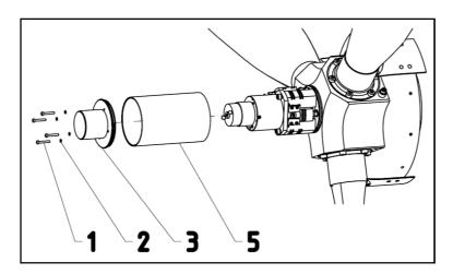
Fig. 5 Removal of covers of electro-mechanics
