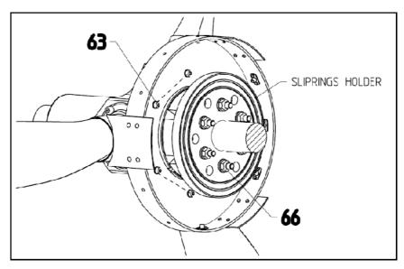
Fig. 2 Rear side of propeller installaed on engine
