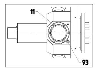
Fig.3 Securing bolts on retention nuts and balance weights
