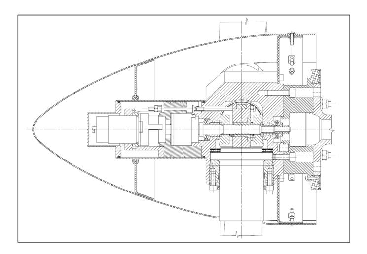
Propeller hub is made of aluminium alloy, and incorporates hydraulic mechanism for adjustment of blade pitch, and blade root pockets. Blades have mixed composition. Precisely machined wooden cores are covered in composite material, and their leading edges are protected by cast polyurethane or stainless steel inserts. Blade roots are set in aluminum alloy ferrules transferring the rotation and centrifugal forces into propeller hub.
