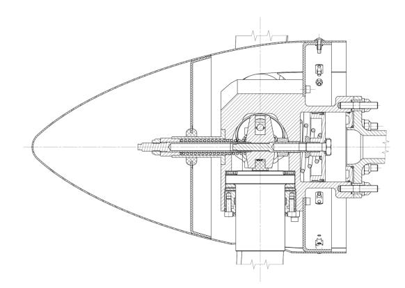
KW-30 family of propellers are designed for aircraft with piston engines coupled with reducing gearbox.
