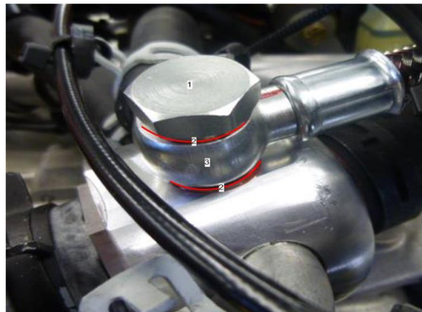
Fig. 11 – Heater supply hose on thermostat: 1-hollow screw 2- copper seal ring 3-ring type nipple
