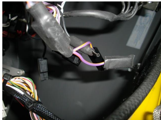
Fig. 4 - Isolation of cable end
