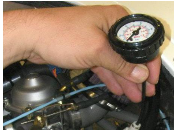
Fig. 4 - Connection between clutch and pressure reducer
