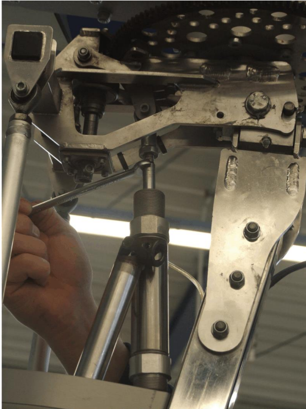
Fig. 1 - Disconnect rod end from ball joint (step 4)
