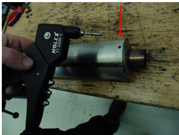
Fig. 6 - Riveting of the outer shell
