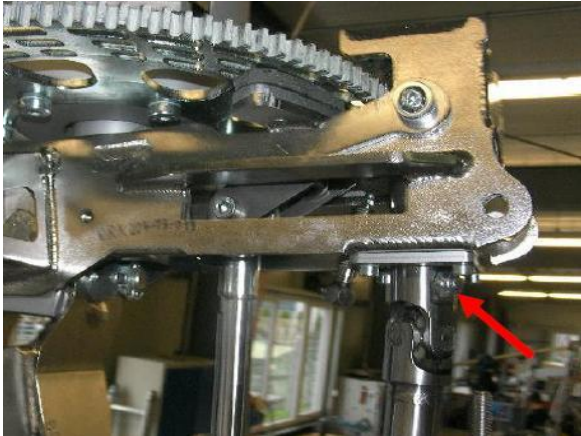
Fig. 1 - Upper pre-rotator drive connected to Bendix shaft
