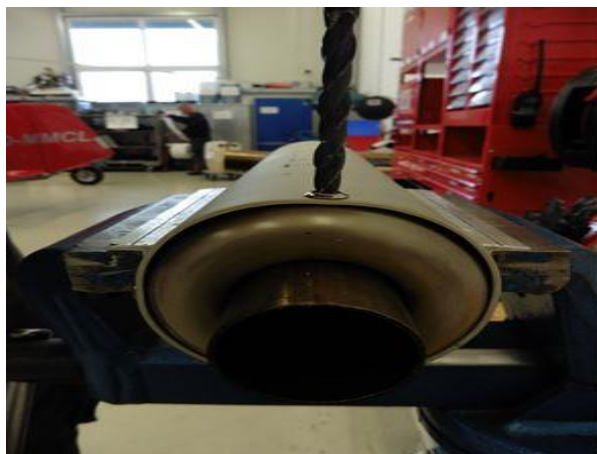
Fig. 3 - Drill out the rivet pin
