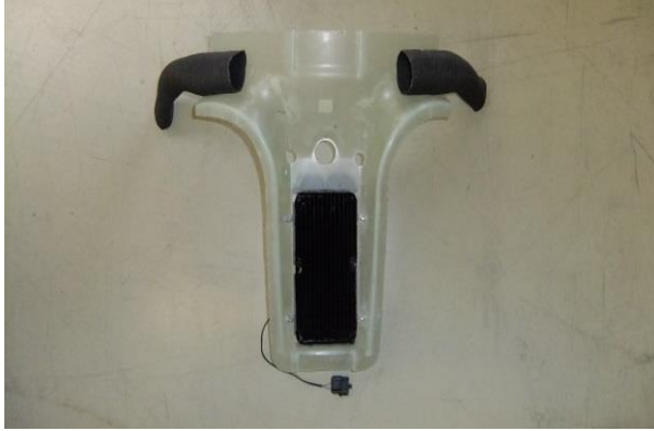
Fig. 1 – Hot-air duct with hot-air hoses
