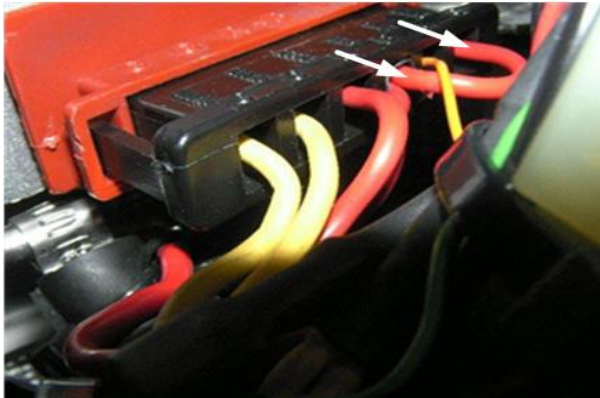
Fig. 1 – Cable connector equipped with rectifier-regulator bridge
