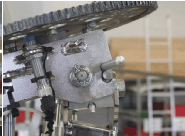
Fig. 3 - Modification of rotor head stop
