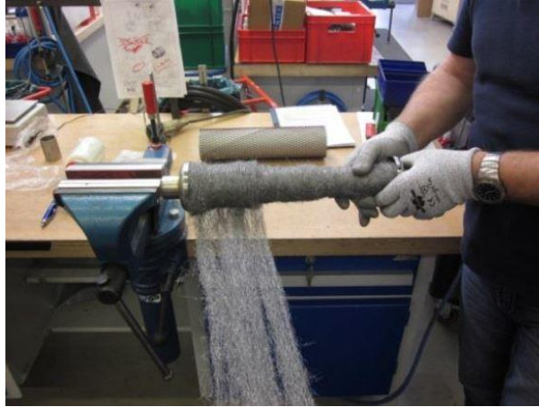
Fig. 4 - Installation of absorption wool
