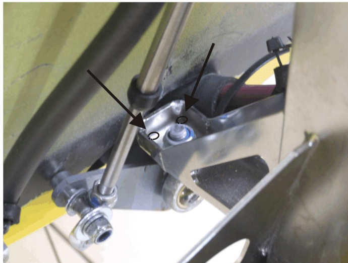
Fig. 1 - Inspection of base control unit attachment
