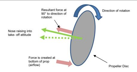
Logically then, to compensate for these effects, an appropriate amount of right rudder must be applied during take-off when applying full-power. The faster the power is applied, the quicker the required pedal input is also required.
