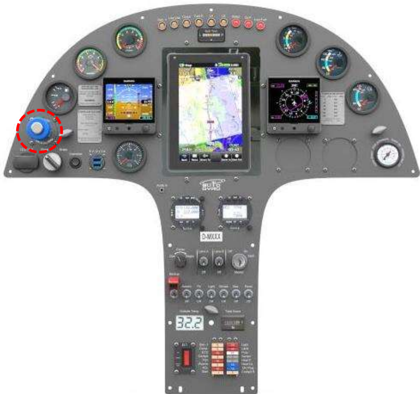
Example of panel from MTO Sport 2017 915iS/916iS with blue propeller control fitted
