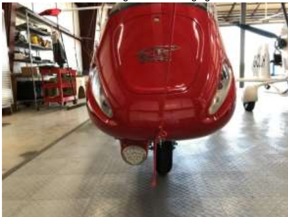
View showing underbody landing light option fitted
