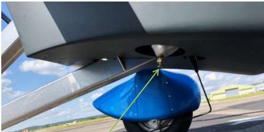
Location of gascolator drain point
