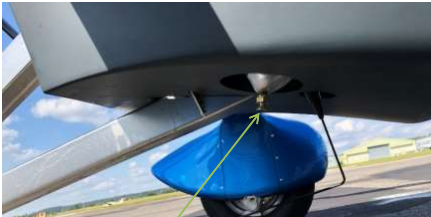
Location of gascolator drain point
