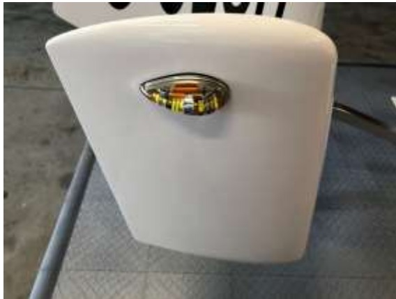
Navigation and strobe units (Aveo certified) fitted to either side of the the tail fins
