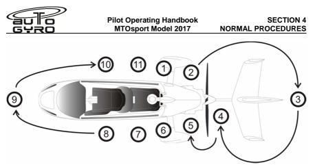
The following checks must be carried out before each flight. However, if the gyroplane is operated by a single pilot or within an organization where the checks are performed by or under the supervision of qualified personnel, check list items marked with a preceding ' $\Theta$ ' may be carried out daily, before the first flight of the day.
