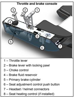
Do not try to disengage the locking pawl by pressing the small release lever without pulling the brake lever at the same time. Releasing the pawl using the small release lever only will lead to premature deterioration of the teeth. If the teeth are worn the function of the parking brake will be compromised!
