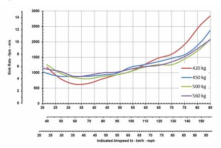
In case of an engine failure, expect a glide ratio of 1:3 which corresponds to a vertical distance of 900 m or 0.5 nautical miles for each 1000 ft.
