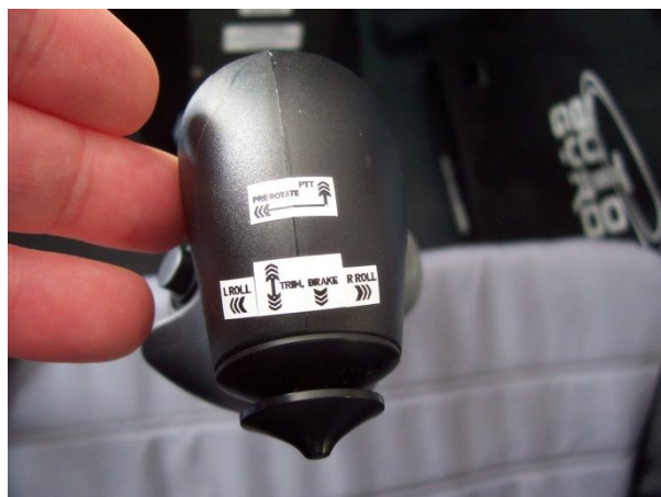
Placard fitment if pitch & roll trim fitted
