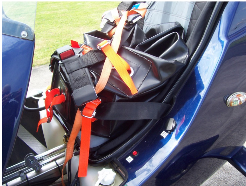
Tank collapsed to 10 litres remaining (Minimum level to ensure that the shape is suitable for retention in the seat)
