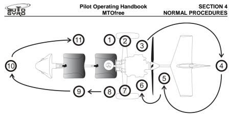
The following checks must be carried out before each flight. However, if the gyroplane is operated by a single pilot or within an organization where the checks are performed by or under the supervision of qualified personnel, check list items marked with a preceding 'O' may be carried out daily, before the first flight of the day.
