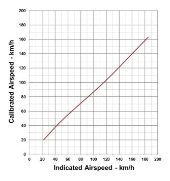
**Example**: Indicated airspeed of 140 km/h represents a calibrated airspeed (corrected for installation error) of 121 km/h.
