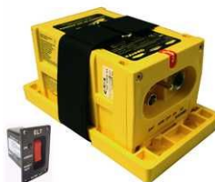
ELT transmitter and cockpit switch
