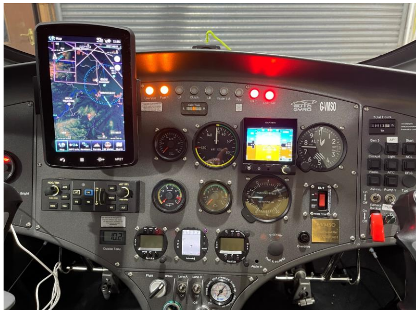
Simple panel installation with Garmin G5, GMC 507, and a portable GPS
