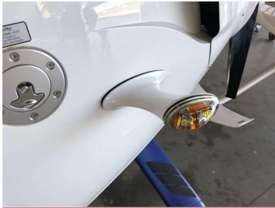
View showing stalk-mounted certified navigation and strobe lamp
