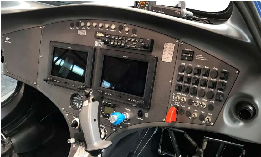
Example of panel from Cavalon 915 with blue propeller control fitted (and dual panel Garmin G3x).
