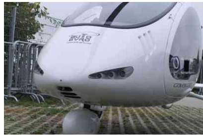
Air intake and gills for condenser
