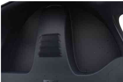
Ducting with cabin air outlets (evaporator behind)
