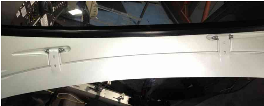
View of the two door hinges. Note direction of bolt fitment.
