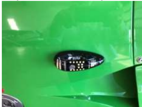
View of uncertified AutoGyro navigation and strobe lamp, for day conspicuity only.
