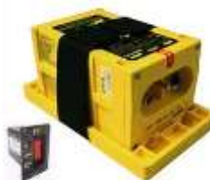
ELT transmitter and cockpit switch
