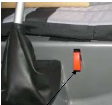
Fuel cock open, and protected by the red cover
