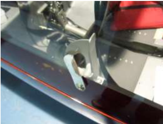
Standard canopy lever (inside/outside)
