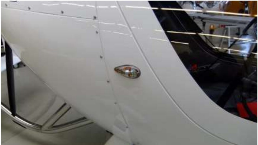
Certified nav and strobe unit, body mounted.
