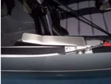
Inside-only lever for semi-open canopy
