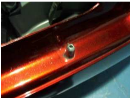
Canopy location spigots and mating holes on the RH side
