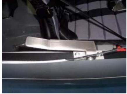
Inside-only lever for semi-open canopy
