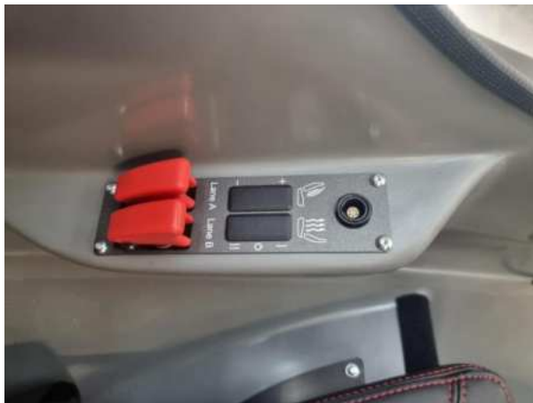
Rear seat headset mounting and seat heating with instructor kill switch option fitted.
