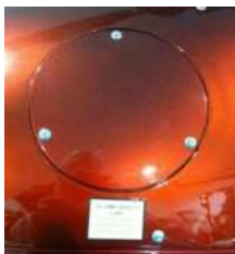
Oil tank access panel
