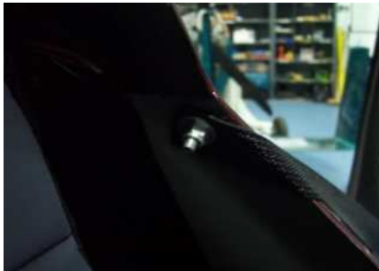
Restraint strap fitting to fuselage (nut cover removed)
