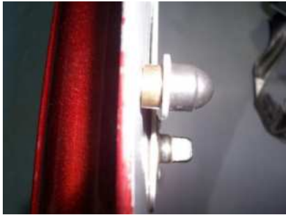
Locking lever pin/bush
