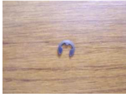
Safety clip fitted at nut-end of hinge pins
