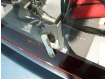
Standard canopy lever (inside/outside)
