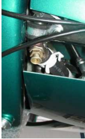
Photo showing water drain point, rear of the suspension bow
