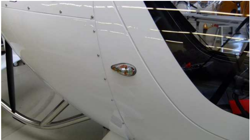
Certified nav and strobe unit, body mounted.
