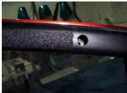
Canopy location spigots and mating holes on the RH side
