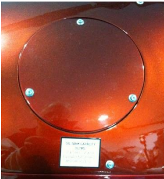
Oil tank access panel
