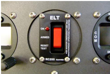
Remote cockpit switch
