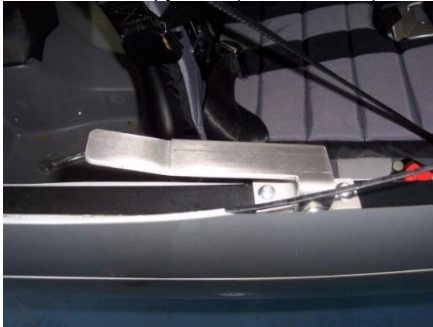
Inside-only lever for semi-open canopy
