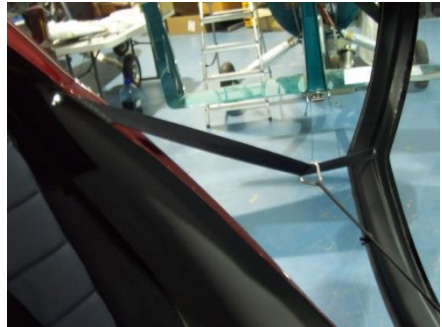
Canopy restraint arrangement
