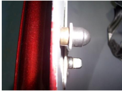
Locking lever pin/bush
