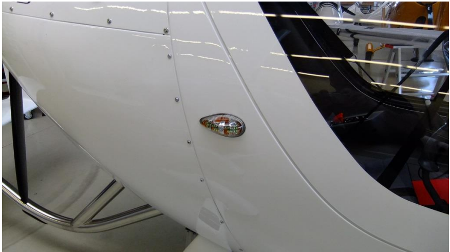
Certified nav and strobe unit, body mounted.
