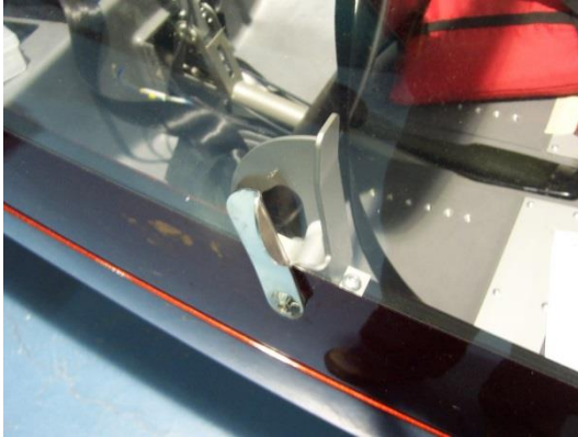
Standard canopy lever (inside/outside)
