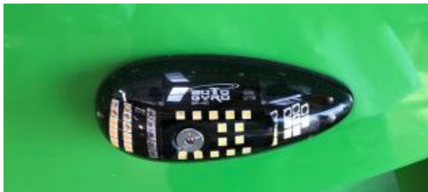
View of uncertified AutoGyro navigation and strobe lamp, for day conspicuity only.
