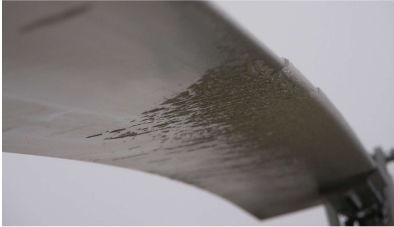
Photo of rotor blade with significant icing built up
