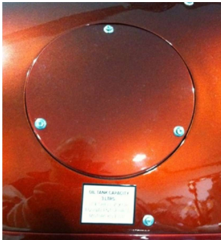
Oil tank access panel
