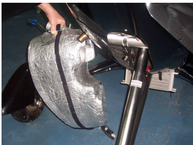
Tank removed from LHS of aircraft
