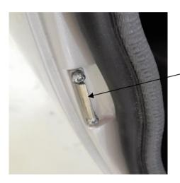
Always check if there is a little bit of grease, vibrations and parts without grease can cause the door opening
