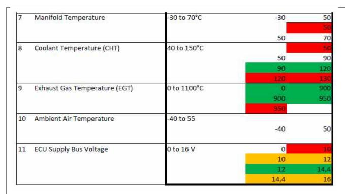
Changes to the indication limits must be recorded within the aircraft documentation, in line with the requirements of the country of operation.
