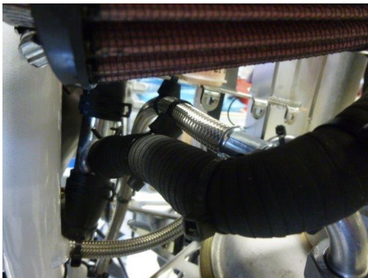
Fig.9: Connection between expansion tank and water distribution pipe with one radiator at the rear of the engine
