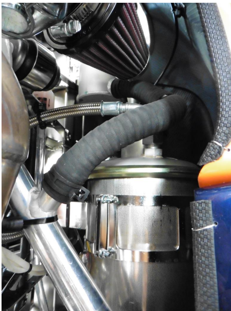
Fig.10: Connection between expansion tank and water distribution pipe with two radiators in side scoops
