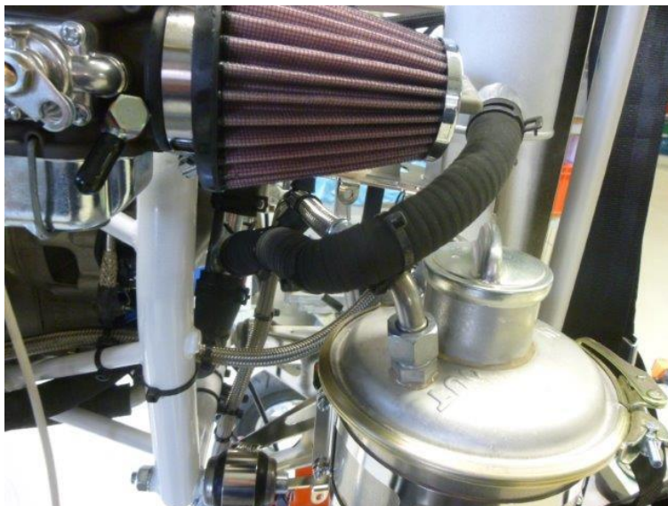
Fig.8: Connection between expansion tank and water distribution pipe with one radiator at the rear of the engine
