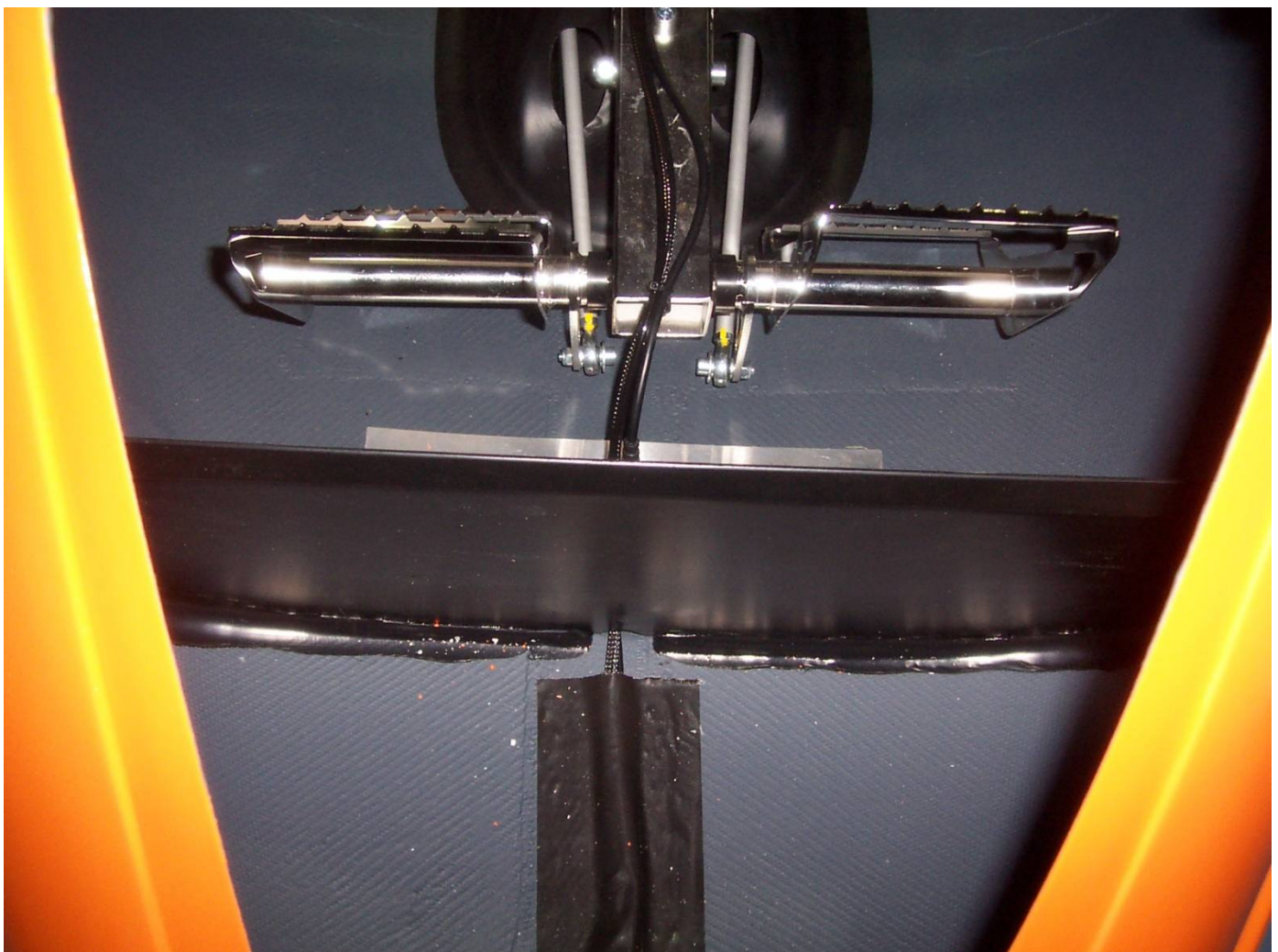
Front pedal installation viewed through nose hatch
