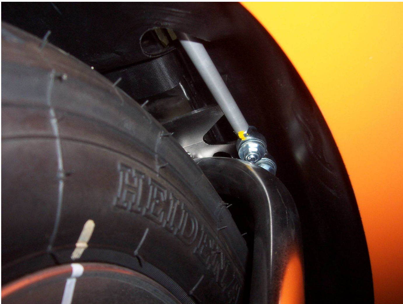
Underside view - pedal connections to nose-wheel fork
