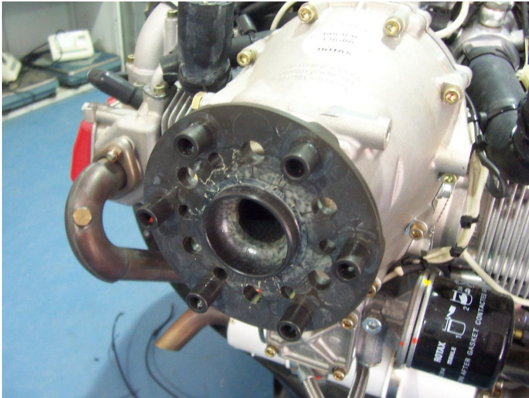
Propeller mounting flange
