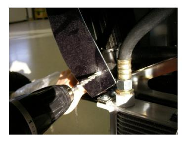
Depending on airframe configuration (MT-03 or MTOS) it may be necessary to use right-angled brackets RSD3045/RSD3046 to attach the enclosure to the oil cooler mounting on the airframe
