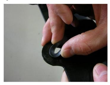
2) Assemble the air scoop/radiator mounts front and rear to the radiator using roundhead M6x12 screws and retaining caps from M.WA07
