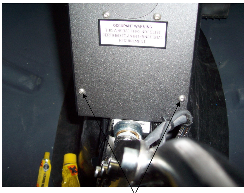
Instrument panel lower mounting screws
