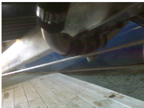
MT-03 installation showing close proximity of rudder cable and P-clip
