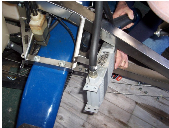
Temporary relocation of the oil cooler to give access for the right-angle drill
