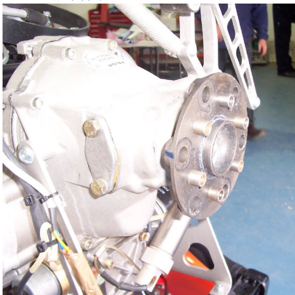
Photo 1, New top hat bushes fitted to flange
