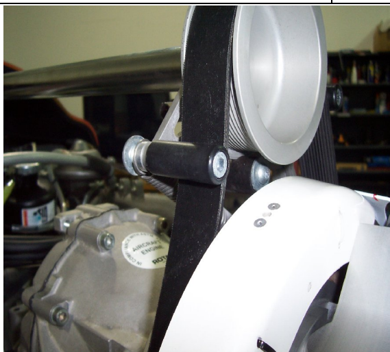
Photo 3, Shorter brake parts to clear prop backing plate
