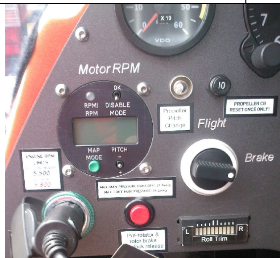
Photo 7, CSC-1/RS controller, LED and C/B in place
