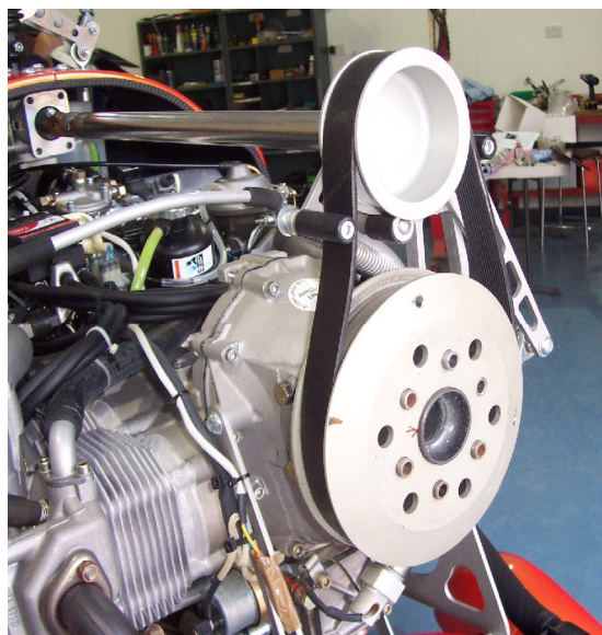
Photo 2, New pre-rotator drum & brake parts fitted
