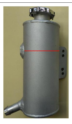
Fig.11: Filling quantity of coolant
