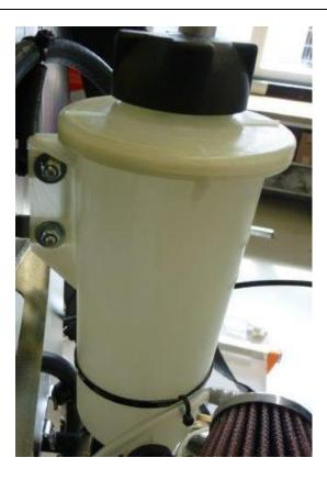
Fig.3: Composite expansion tank II
