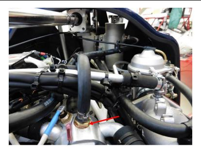
Fig.7: Connection between expansion tank and highest point
