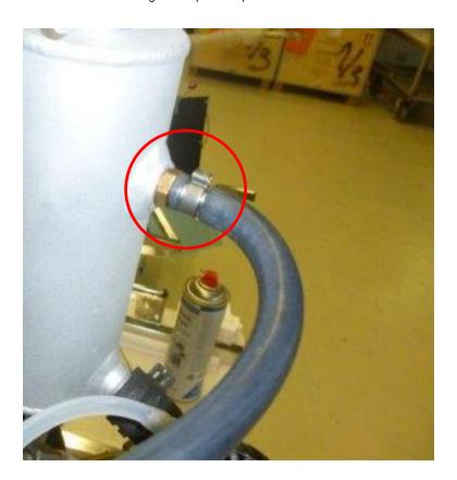
Fig.4: Nipple with copper washer and crimp
