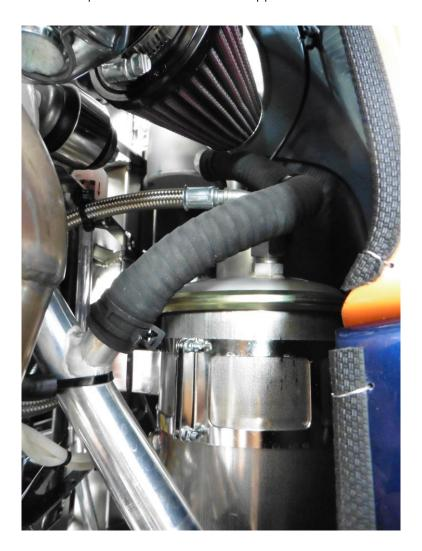
Fig.10: Connection between expansion tank and water distribution pipe with two radiators in side scoops
