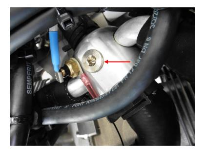
Fig.1: Dummy plug
