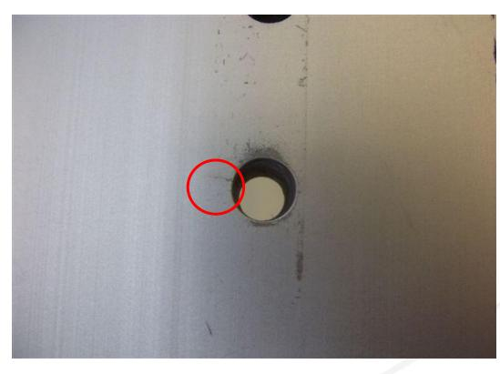
Example for occurring cracks from the bore hole on two sides approx. 30mm
