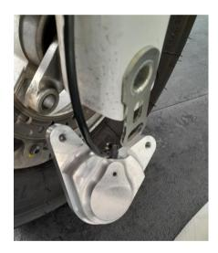
Remove the brake piston from the caliper, either by using the brake lever or using compressed air pushed through the vent screw hole.
