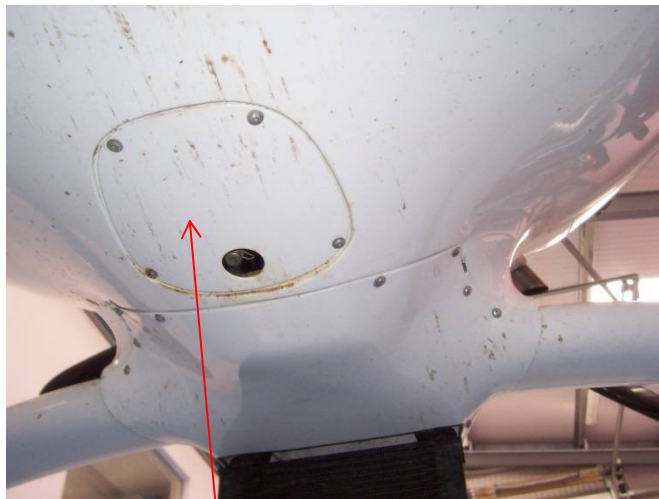
Fig 1 Fuel drain inspection cover
