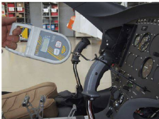
Fig 3 Force gauge to measure stick load
