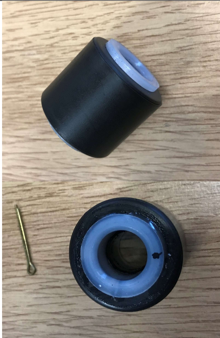
Photo showing the brass split pin and the float with the marked dot (which is fitted uppermost)
