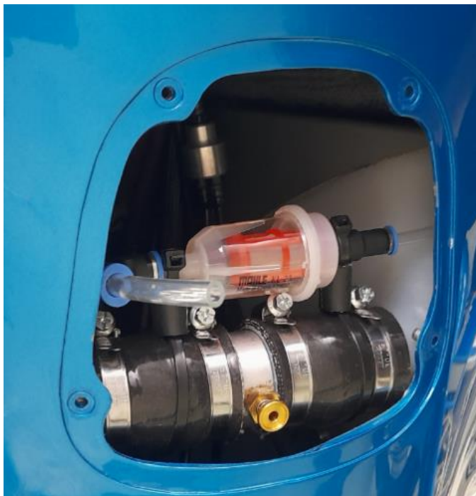
Figure 31: Re-positioned vent line with filter
