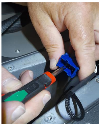
Figure 6-12: Disconnect plug, remove safety lock, pin out the fuel level sensor
