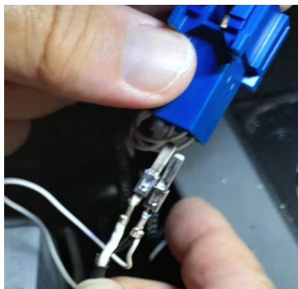
Figure 6-12: Disconnect plug, remove safety lock, pin out the fuel level sensor
