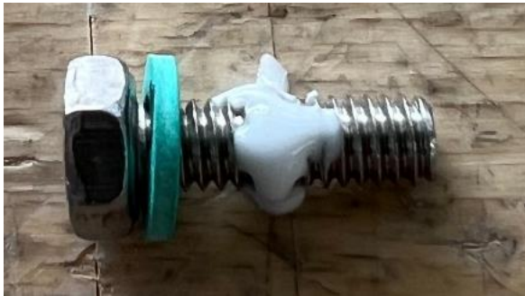
Picture 32: Loctite application on thread of lid screws. Do not put it on the end of the bolt or on the mating part; this drives sealant through the nut and into the tank.
