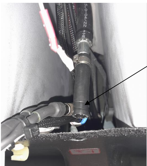
Figure 25: Hoses disconnected from old Shut-off valve
