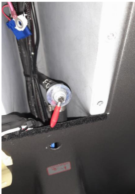
Figure 24: Fuel Shut-off valve nut removed
