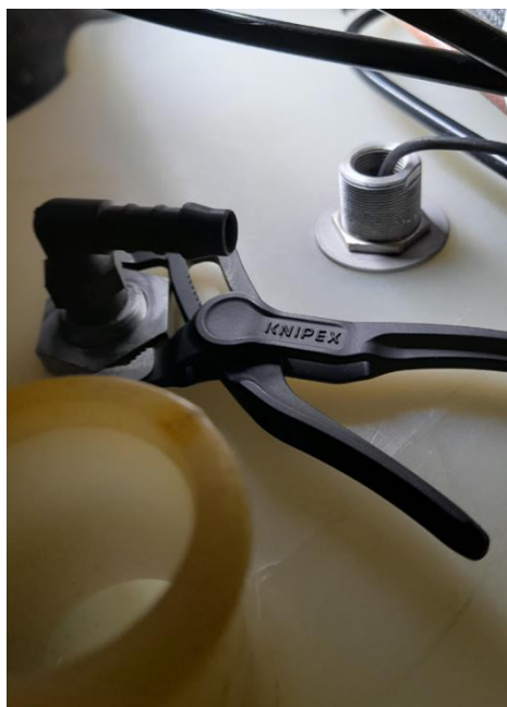
Figure 23: use small water pump tongs or equivalent to tighten new assembly
