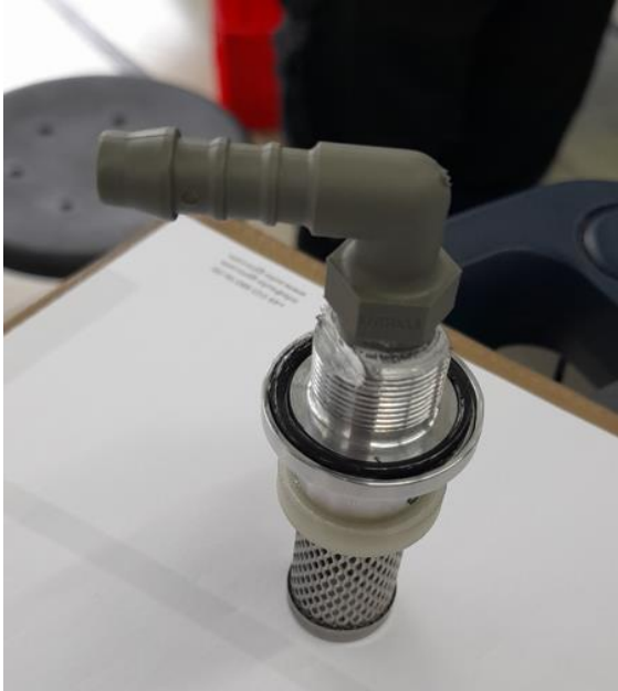
Figure 22: new fuel take-off with greased O-ring
