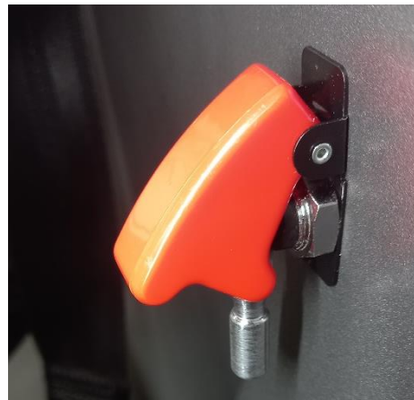
Figure 27: lever installed, open = vertical
