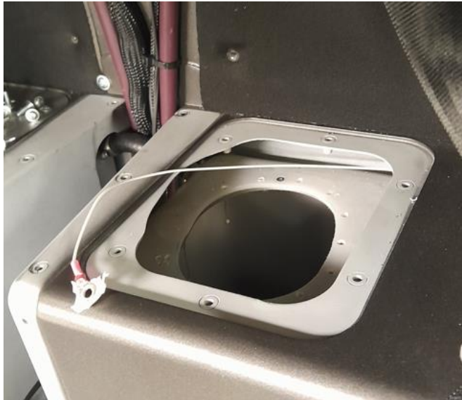
Figure 13: Fuel level sensor removed
