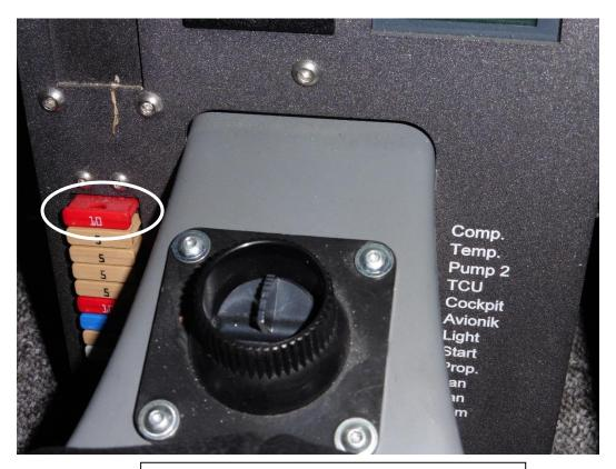
Fig. 1: 10A Fuse Compressor
