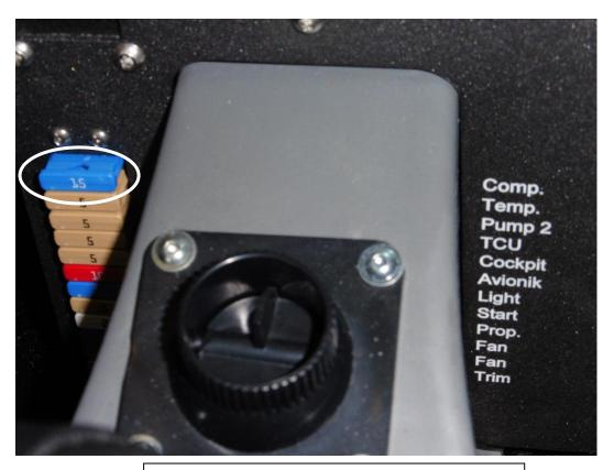
Fig. 2: 15A Fuse Compressor
