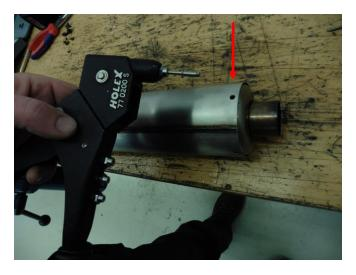
Fig.5: Riveting of steel tube
