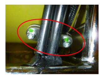
Fig.3: Screw locking varnish
