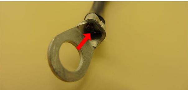
Fig. 1 – Inaccurate crimp connections
