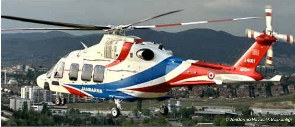
The first T625 GÖKBEY Helicopter with tail number J-6001, en route to the Gendarmerie Aviation Department premises in Güvercinlik, Ankara. The first 3 GÖKBEY Helicopters, expected to be delivered by the end of 2023, are designated as T625J due to their weight being approximately 250 kg heavier than the remaining 17 helicopters scheduled for serial production
