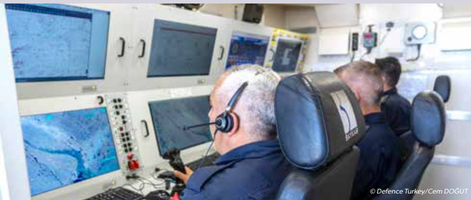
A snapshot from inside the Ground Control Station of the BAYRAKTAR TB2 Armed UAV: The Mission Commander is in the center, the UAV Pilot on the right, and the Payload Operator on the left are seen carrying out their tasks
