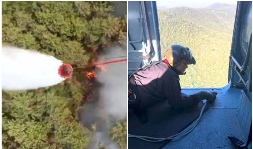
Above: During Forest Fire Suppression Operations, Technicians hanging out of the doors of Mi-17 helicopters ensure precise water drops with the Bambi Bucket by observing the fire from above. Below: A Mi-17 Helicopter is flying towards a nearby reservoir to collect water using the Bambi Bucket.
