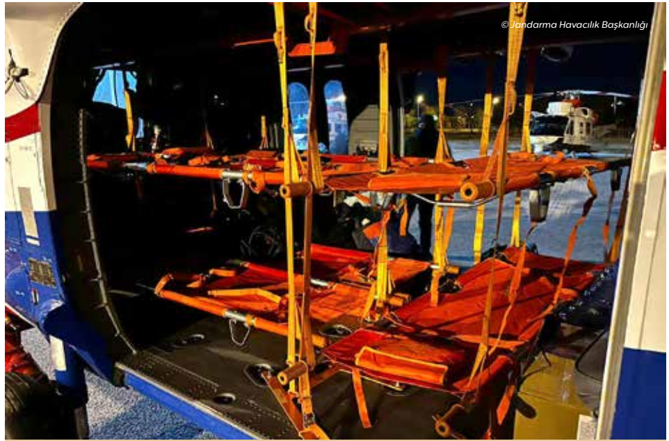
The portable stretchers that can be mounted on the Gendarmerie S-70i Utility helicopters provide the capability for airborne medical evacuation of up to 8 individuals
