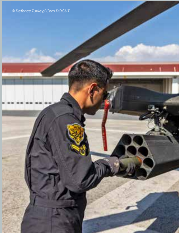
© Defence Turkey/ Cem DOGUT Loading of 70mm Unguided Rockets onto the T129 ATAK Helicopter
