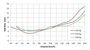
In case of an engine failure, expect a glide ratio of 1:3 which corresponds to a vertical distance of 900 m or 0.5 nautical miles for each 1000 ft.
